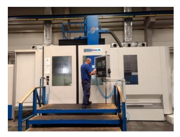
Another significant investment in ZKL Brno, a.s. in 2019 was the acquisition of a new centerless grinder **BB 400ST CNC** in the hall 4. This grinder, allowing grinding of elements within the diameter range of 50 to 250 millimetres, has significantly expanded the existing capacities for grinding rolling element casings in the segment of large-scale bearings.
