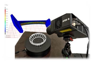
In ZKL, we are now using the semi-automatic system ATOS Q for comprehensive metrology, especially for complex-shaped components such as various types of bearing cages. This system is designed for industrial use and provides fully traceable measurement results even in challenging conditions. Its optics and electronics are protected against dust and splashing water, allowing the scanner to be used both in the laboratory and on the production floor for quality control purposes.
