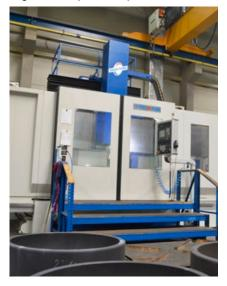
gives it the opportunity to machine parts up to 2000 mm in diameter and up to 12 tonnes in weight. Modern control system Sinumerik 840D SL and other Siemens electronics ensures precision machining of complex shaped parts. Machining tools are stored in a twelveslot magazine and, after an automatic exchange, they are measured automatically by an integrated Renishaw tool probe.
