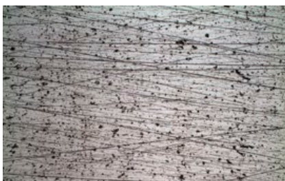
Marks from manufacturing residues—small, irregular indentations and scratches.
