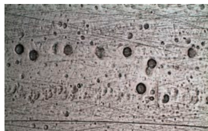
Imprints on a bearing part surface caused by equally sized process contaminants.
