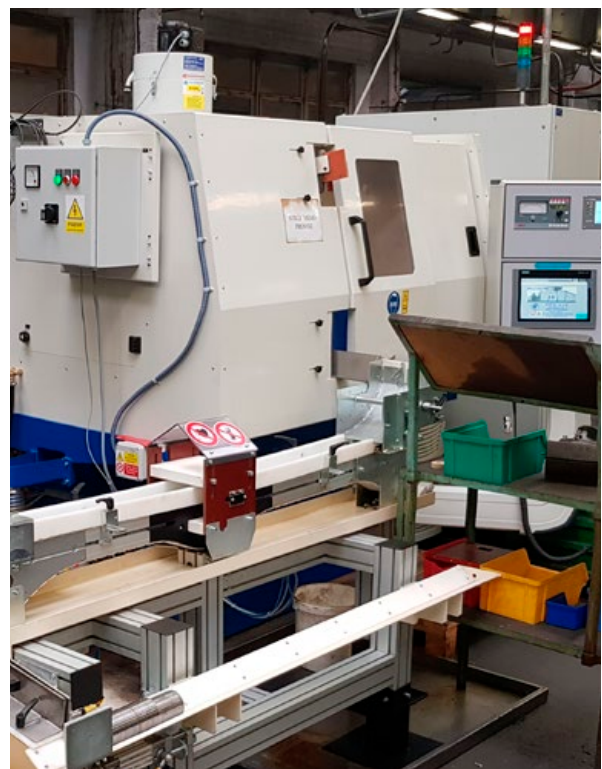
Installation of a machine for precise grinding of BDLZ 120 CNC HP arms
